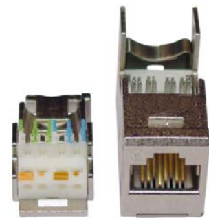
Figure 6: E-DAT Field Termination Module with RJ45 to Insulation Displacement Connectivity (IDC). T568A Wire Color Code shown here. Shield Connectivity Spring Provides Equipotential Bonding to DIN Rail Grounding Clips (see Figure 4).
